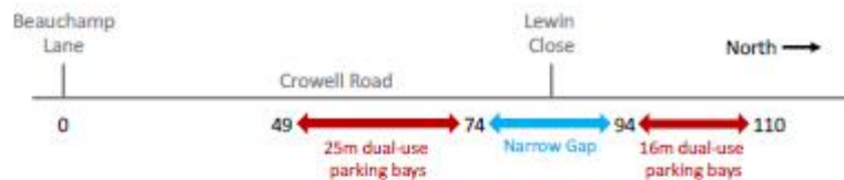
Figure 1. Schematic drawing of the location of the proposed dual-use parking bays in relation to the entrance of Lewin Close. All roads are coloured dark grey with Crowell Road running from left (South) to right (North). The north-eastern kerb line of Beauchamp Lane is marked on the left of the line representing Crowell Road. The proposed dual-use parking bays are marked in red, whilst the narrow gap with less than 3m distance from the entry to Lewin Close is marked blue.
